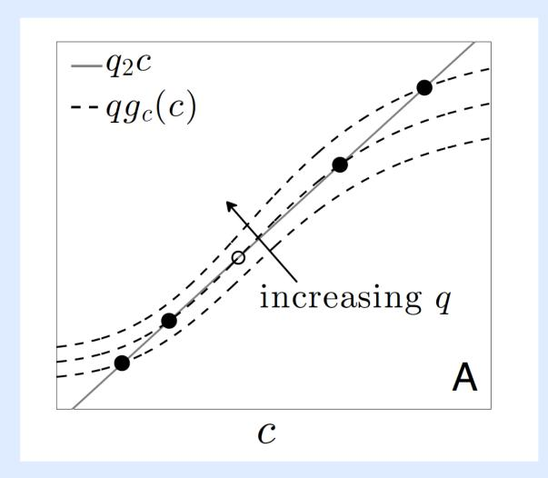
$0 = qg_c(c) - q_2c$ One (stable) or three (two stable, one unstable) intersections depending on q
