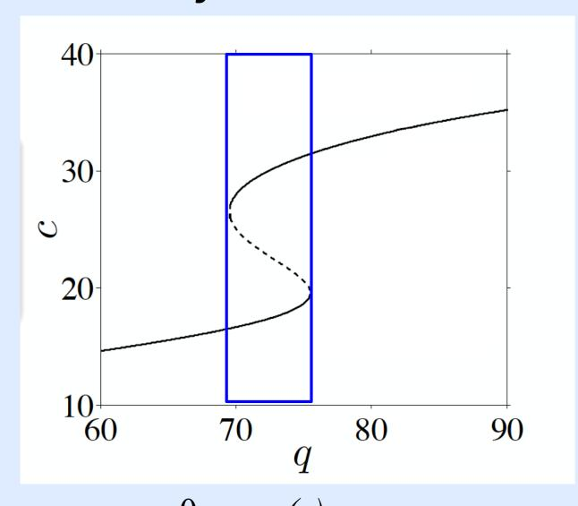
$0 = qg_c(c) - q_2c$  *q* bifurcation parameter controlling fast flow at short time
